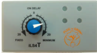
Figure 3: Optional On-delay timer is adjustable between 0 and 20 minutes in either of fixed or minimum delay. This option also manages the outlets powering sequence in 30 seconds steps.
