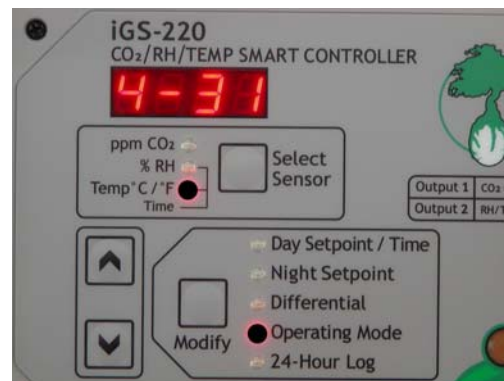
Example :4-31.cooling during the day only and when CO2 (Output 1) is OFF
